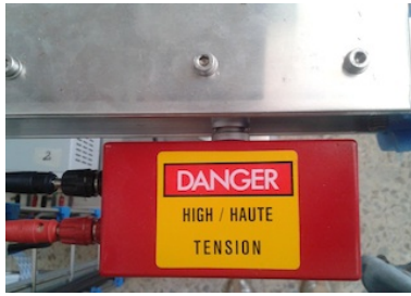
Fig.14 Box connected to MRPC by +HV connector
