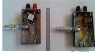
Fig. 4 HV box red and blue, respectively for positive and negative voltage
