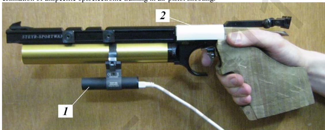
Figure 1. The air-pistol during an experimental shot: 1 is SCATT system sensor; 2 is a special shield to hide cocking lever.
