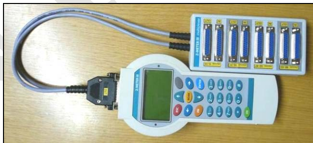
Fig. 2. Z-meter device with external multiplexer
