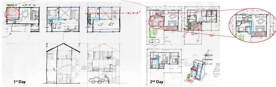
Fig. 6. Movement of rooms toward south (red line) and application of a sliding door (blue dotted line)
