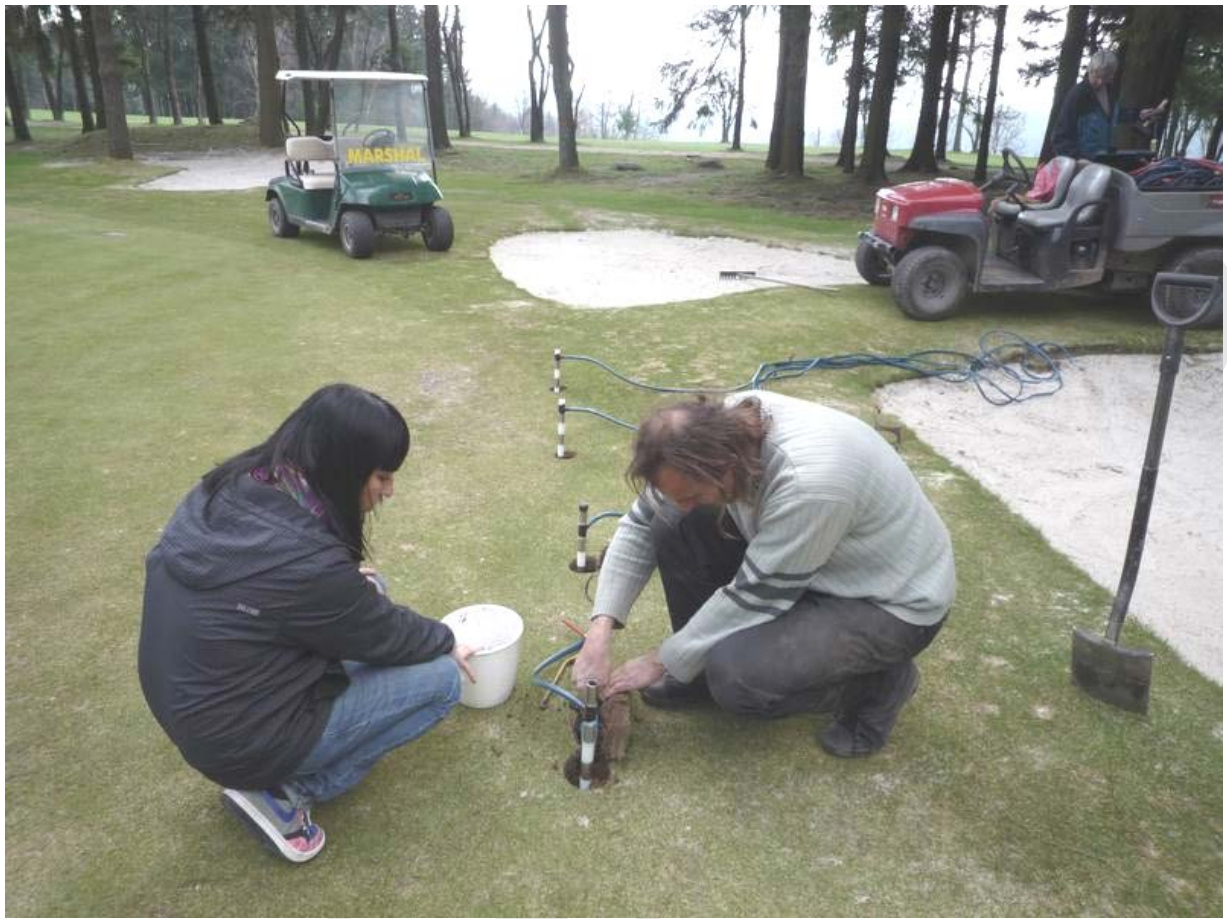
Fig. 5. Installing the probes into monitoring wells on the golf course together with student from Spain
