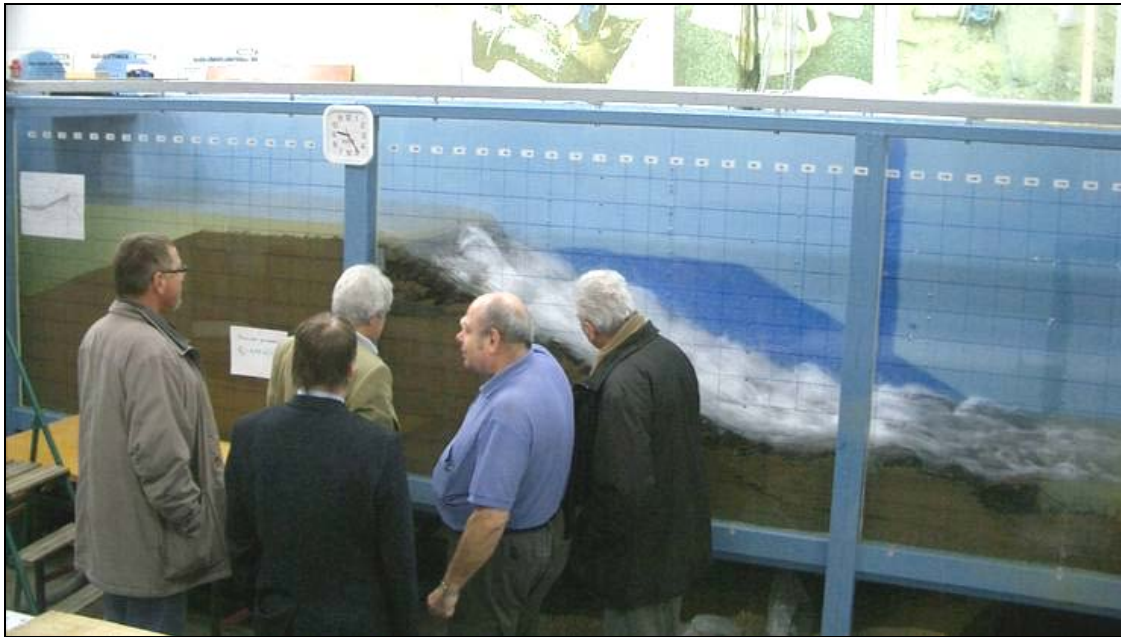
Fig. 4. The applied research for practitioners (hydraulic model of safety spillway polder Žichlinek, M_1 = 10 )
