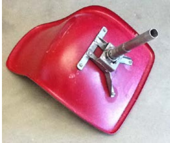
Figure 2. The challenge was to design a base for salvaged seats, recuperated during the renovation of university amphitheatres. The model is inspired by a famous chair designed by Charles and Ray Eames in the 1950's.
